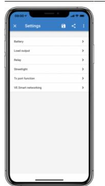
The settings page is accessed by clicking on the Cog icon at the top right of the Home page. The settings page provides access to view or change the settings of the Battery; Load; Streetlight; and Port functions. From this page you can also view Product information such as the Firmware versions installed on the MPPT Solar Charger.
